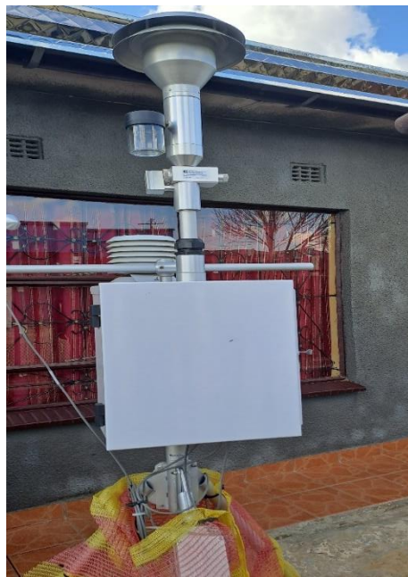
Figure 4: E-Bam instrument commissioned at House 5
