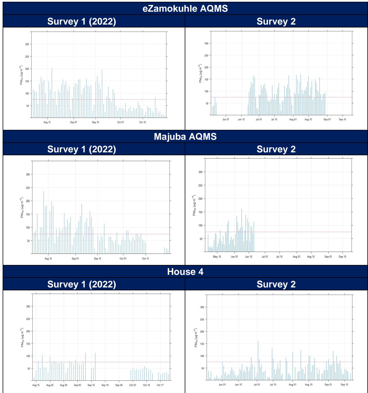
Figure 20: Daily ambient PM_{10} concentrations ( \mu g/m^3 ) measured at the sampling sites during the two sampling surveys.
