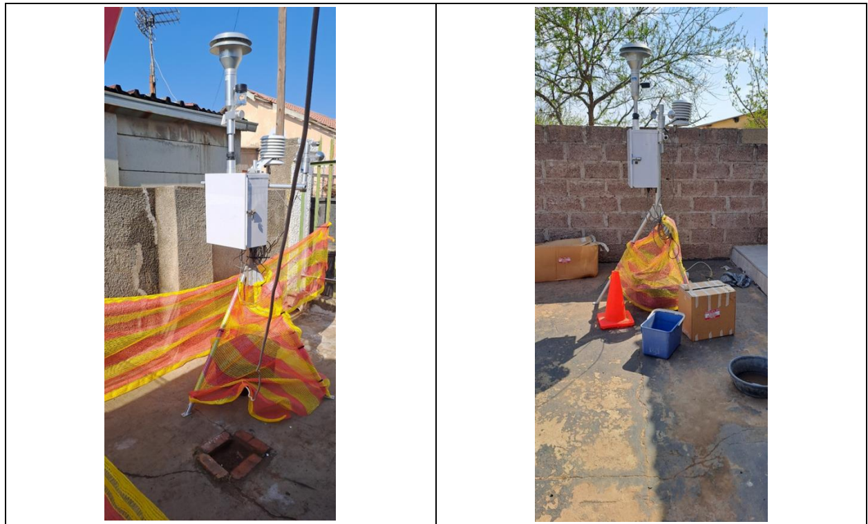
Figure 4: E-Bam instrument commissioned at House 2 (left) and House 5 (right).
