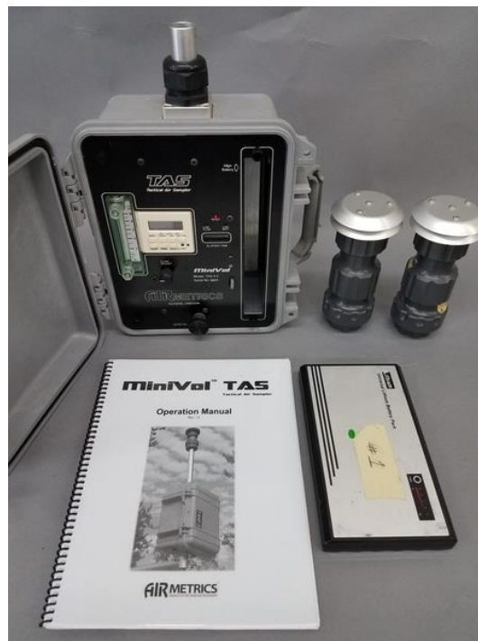
Figure 5: MiniVOL Portable Air Sampler
