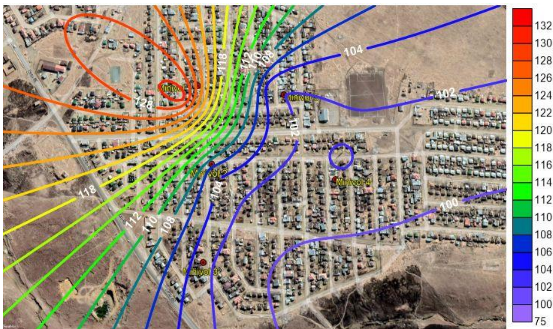
Figure 21: Isopleth map showing spatial distribution of measured PM 10 concentrations in µg/m 3 for 16 th August 2021
