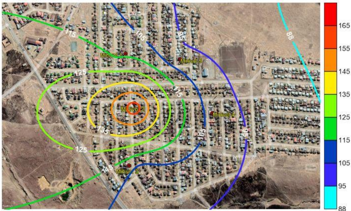
Figure 16: Isopleth map showing spatial distribution of measured PM 10 concentrations in µg/m 3 for 11 th August 2021
