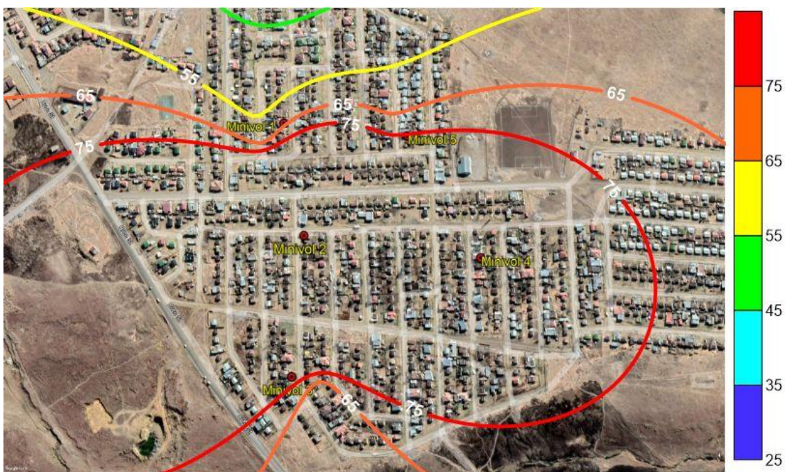
Figure 19: Isopleth map showing spatial distribution of measured PM 10 concentrations in µg/m 3 for 14 th August 2021
