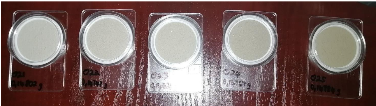
Figure 13: Colour variation of collected filter samples for the same day of sampling
