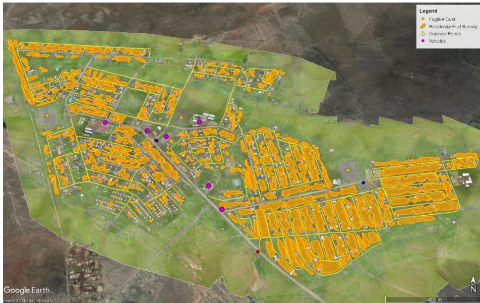
Figure 13: Emission source categories identified in Ezamokuhle based on a ground and aerial based assessment (ARM, 2021b)
