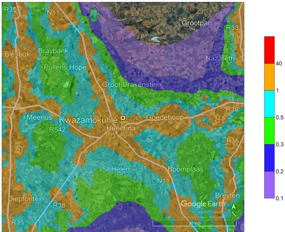
Figure 5-72: Model predicted annual NO 2 ambient concentrations in µg/m 3 for the Vehicles – Paved Roads emission source category within the Greater KwaZamokuhle Airshed
