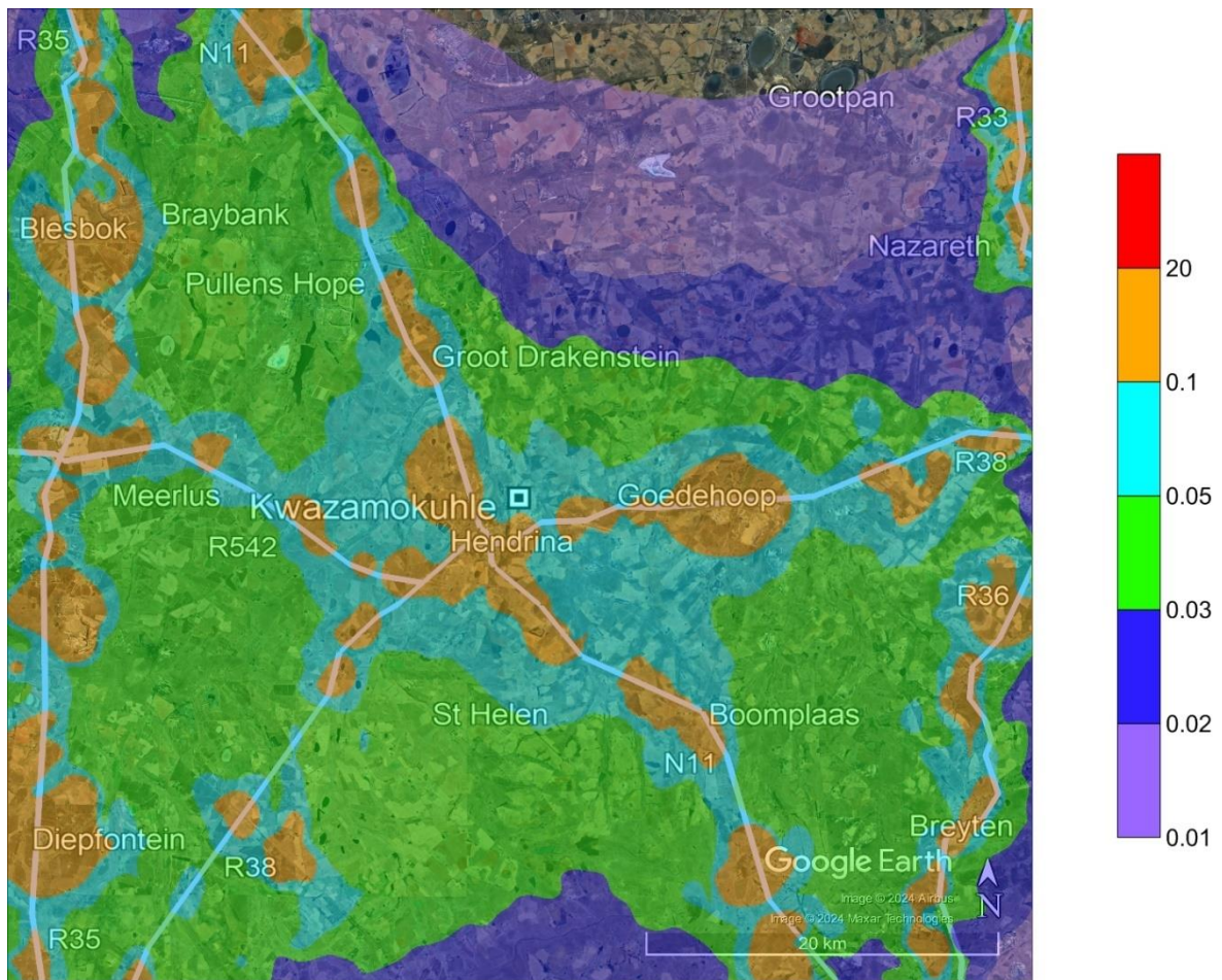
Figure 5-136: Model predicted annual PM 2.5 ambient concentrations in µg/m 3 for the Vehicles – Paved Roads emission source category within the Greater KwaZamokuhle Airshed
