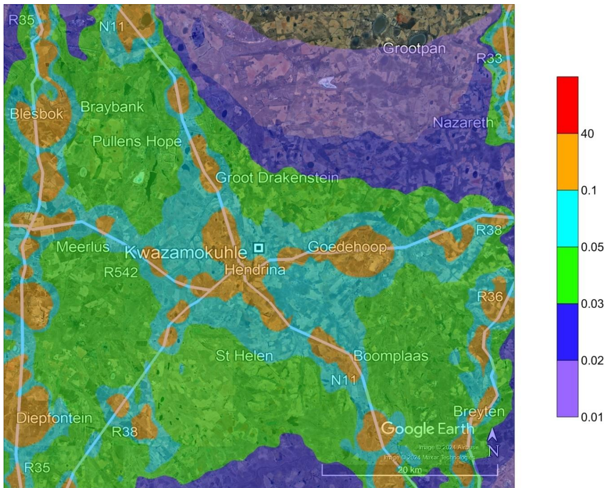
Figure 5-104: Model predicted annual PM 10 ambient concentrations in µg/m 3 for the Vehicles – Paved Roads emission source category within the Greater KwaZamokuhle Airshed
