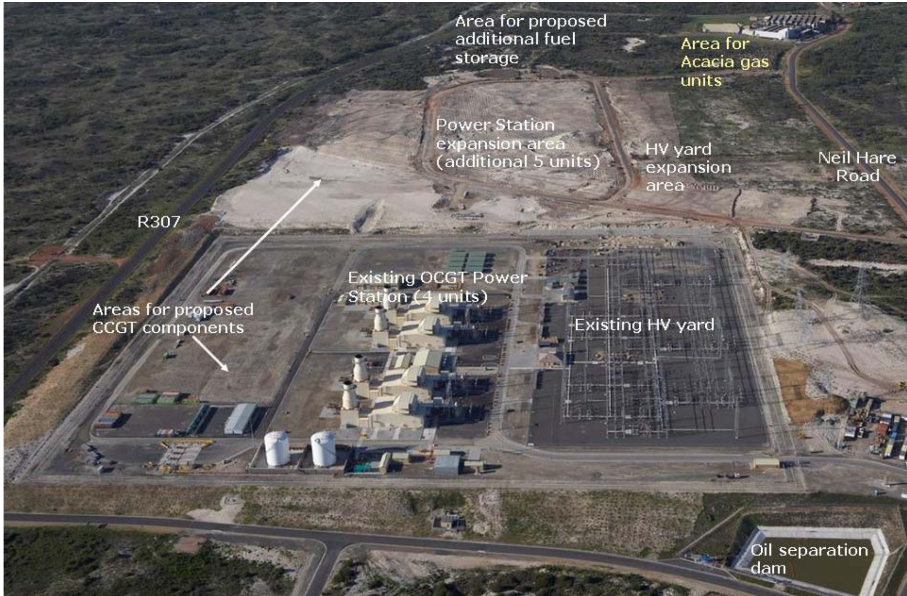
Figure 5.3: Aerial photograph showing the existing Ankerlig Power Station units, the proposed power station conversion and the area proposed for the Acacia and port Rex aero derivative gas turbine units
