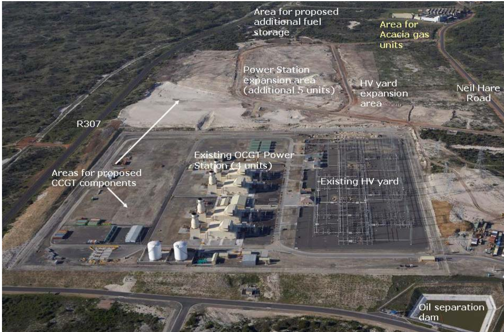
Figure 2.1: Aerial photograph showing the existing Ankerlig Power Station units, the proposed power station conversion and the area proposed for the Acacia and Port Rex aero derivative gas turbine units
