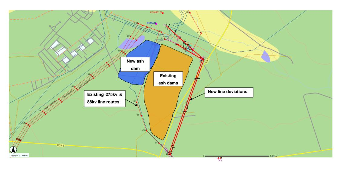
Figure 10: Preferred Route for the Deviation of the 275 kv and 88kv Powerlines at Komati Power Station (TAP, 2007).
