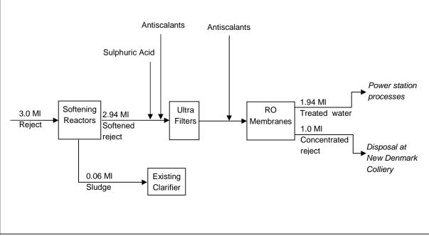
Figure 2.3 Process flow diagram of the proposed reject treatment plant (volume per day)
