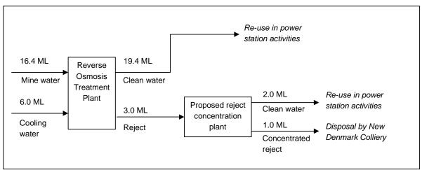
Figure 2.2 Process flow diagram of daily proposed reject treatment and disposal
