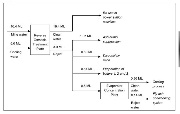
some 1 MI per day. Evaporation is conducted continuously when the unit is operating at a load of greater than 380 MW.
