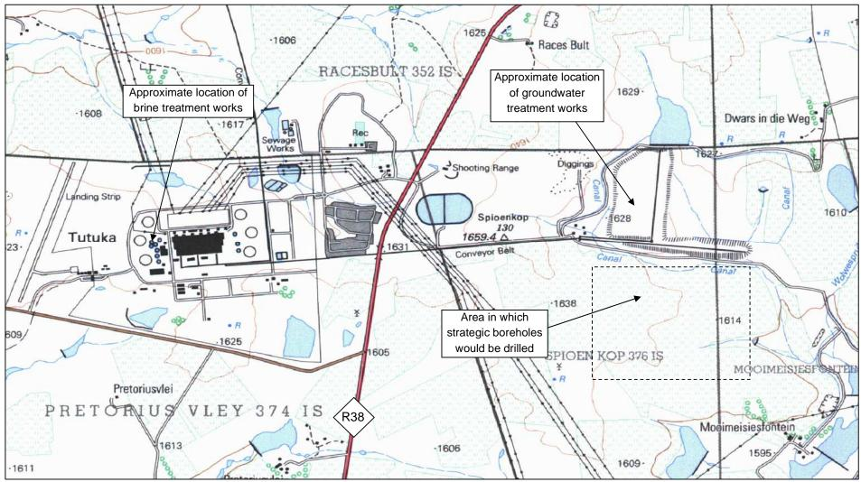
Figure 1.1 Location of the Tutuka power station and proposed treatment facilities (2629 CD)
