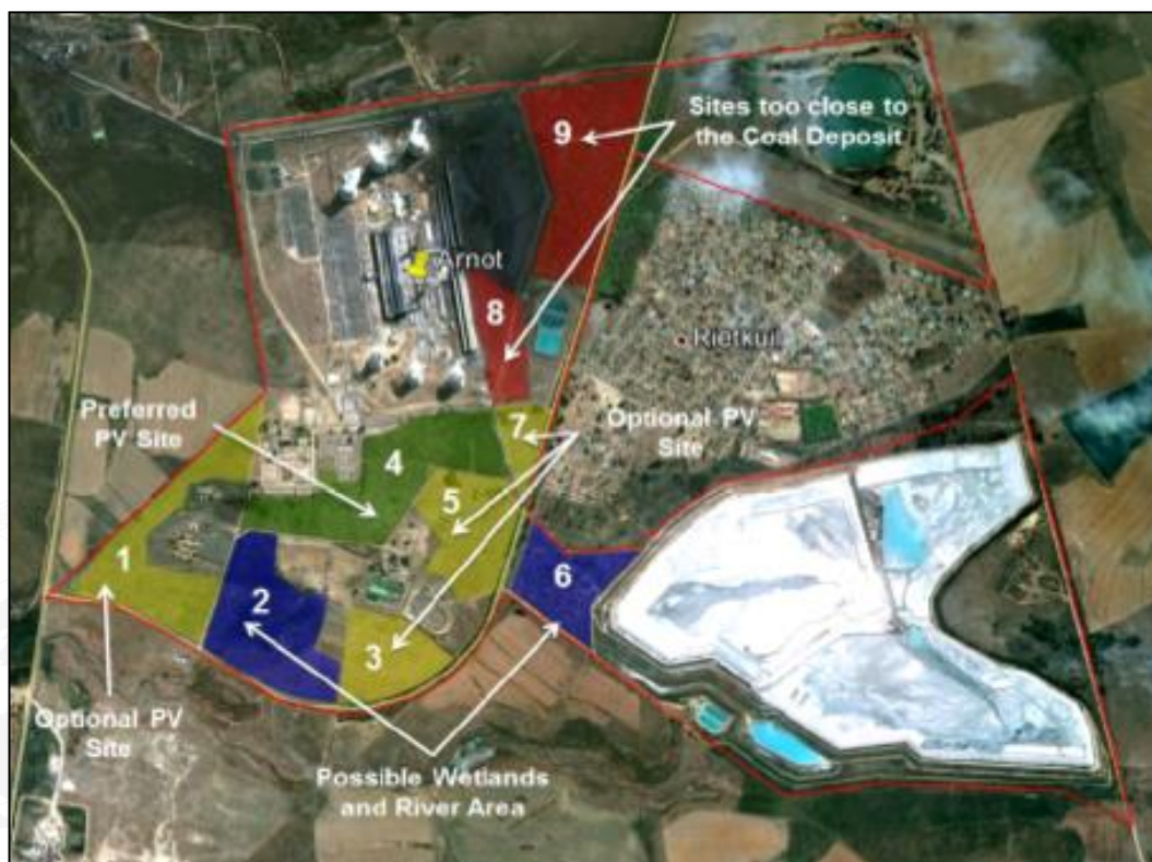
Figure 10: Arnot Power Station Site layout Alternatives (Arup, 2013)
