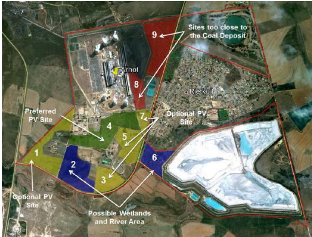
Figure 2: Aerial view of Arnot Power Station with areas of identified possible PV sites
