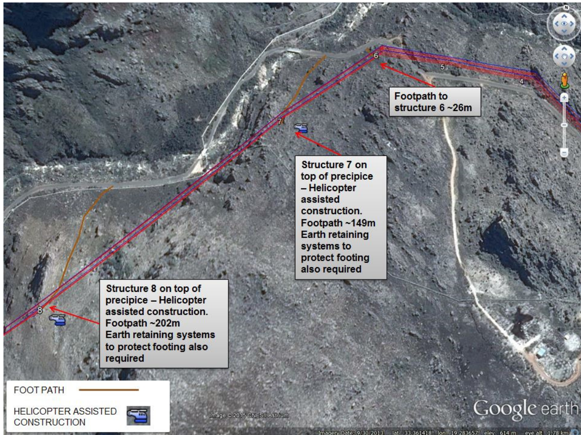
Figure 3-6: Access and construction requirements structures 6 to 8
