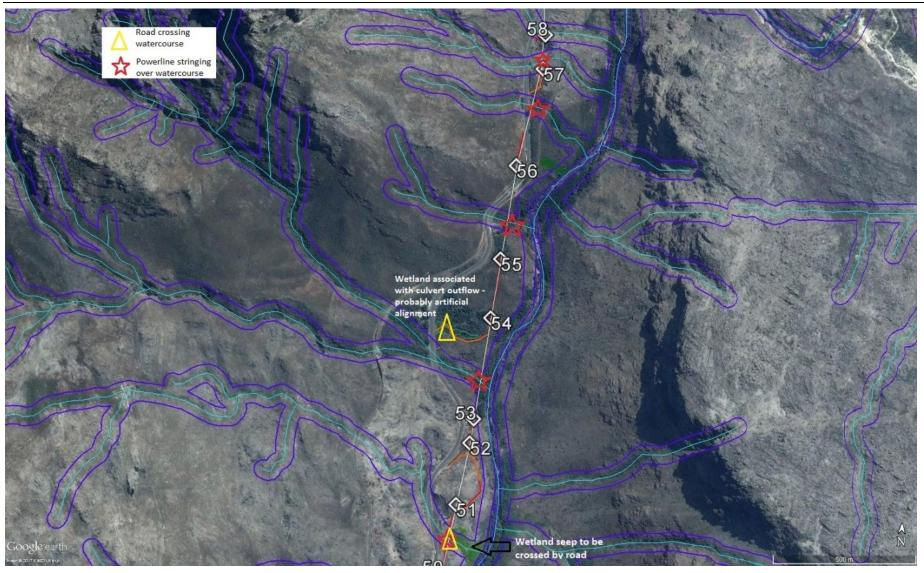
Figure 22 Mitigation recommendations for area between poles 51 and 58 To be read in conjunction with mitigation measures outlined in Section 4 for these areas
