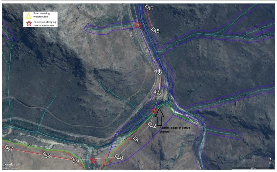
Figure 20 Mitigation recommendations for area between poles 37 and 46 To be read in conjunction with mitigation measures outlined in Section 4 for these areas. Green line indicating active channel roughly delineated.
