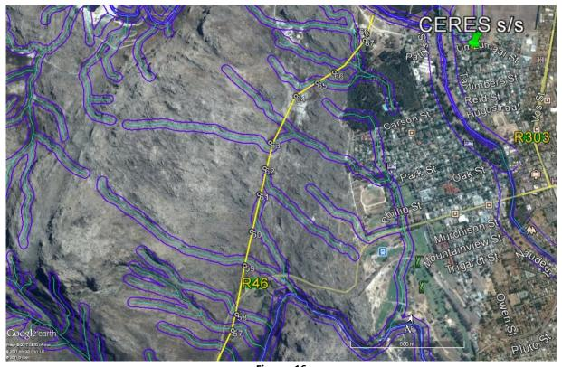
Figures 16 Close view of CESA watercourses between the Ceres substation and proposed pole 57. Buffered watercourses are shown here.
