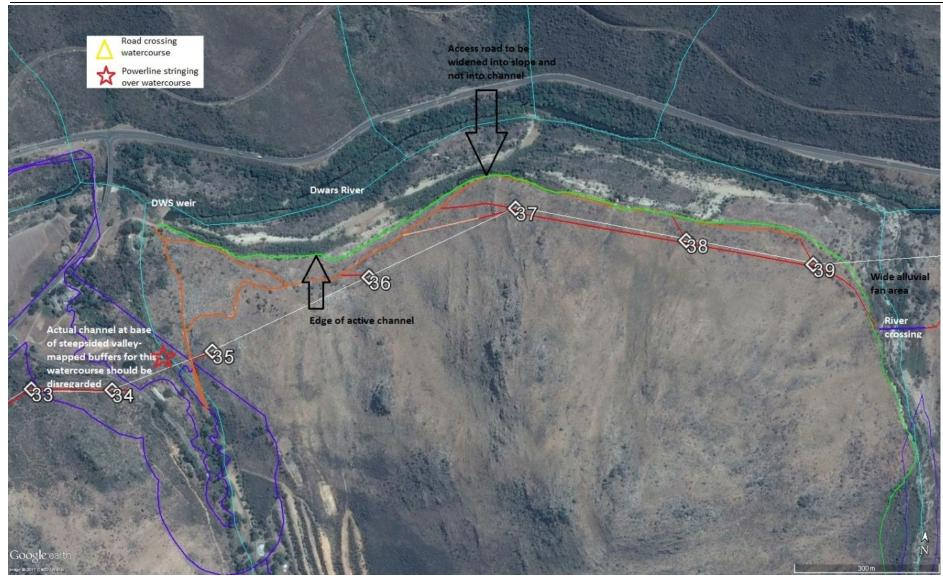
Figure 19 Mitigation recommendations for area between poles 33 and 39 To be read in conjunction with mitigation measures outlined in Section 4 for these areas. Green line indicating active channel roughly delineated.
