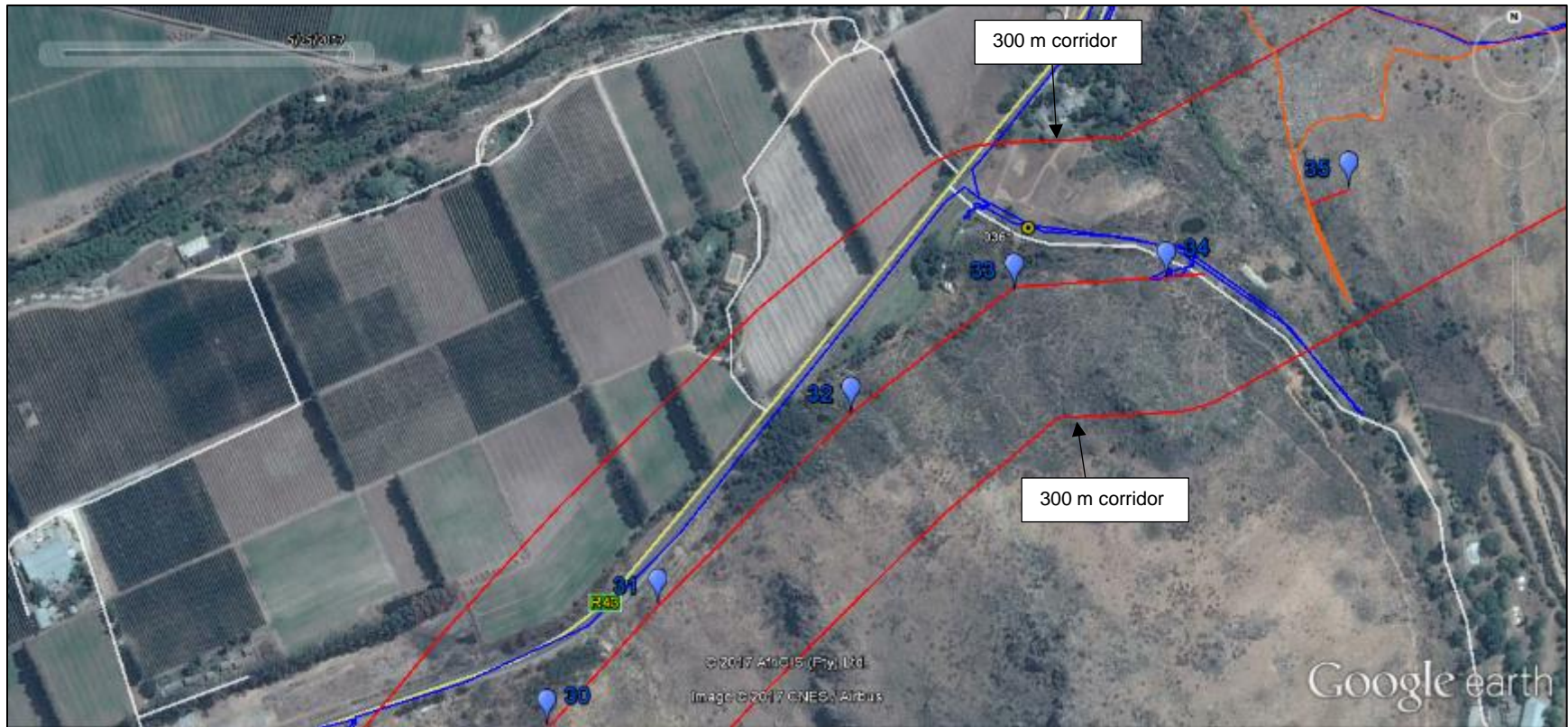
Figure 6.8.1. SURVEY MAP: Google Earth™ aerial image showing 300 m corridor (outer two parallel red lines) for the proposed 132/66kV powerline showing waypoint 0361 (numbered yellow circle icon), proposed tower locations 35 to 30 (numbered blue balloon icons) and proposed access road (red lines = new roads; orange line = old, existing roads requiring upgrading). The survey tracks are indicated by the blue lines.
