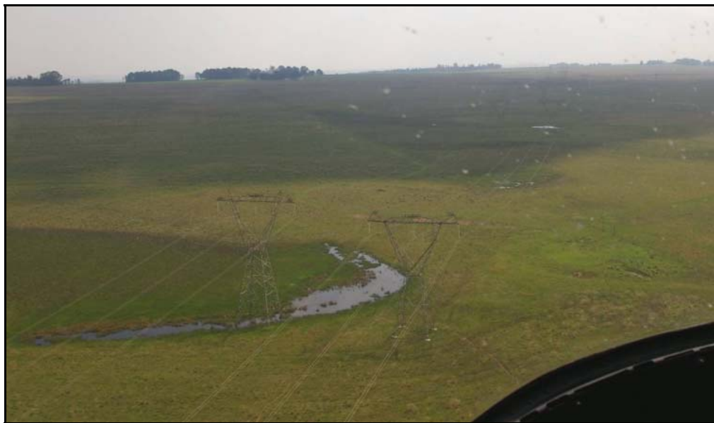
Figure 23: An example of seepage zones being crossed by existing transmission lines in the Hendrina-Prairie portion of the route
