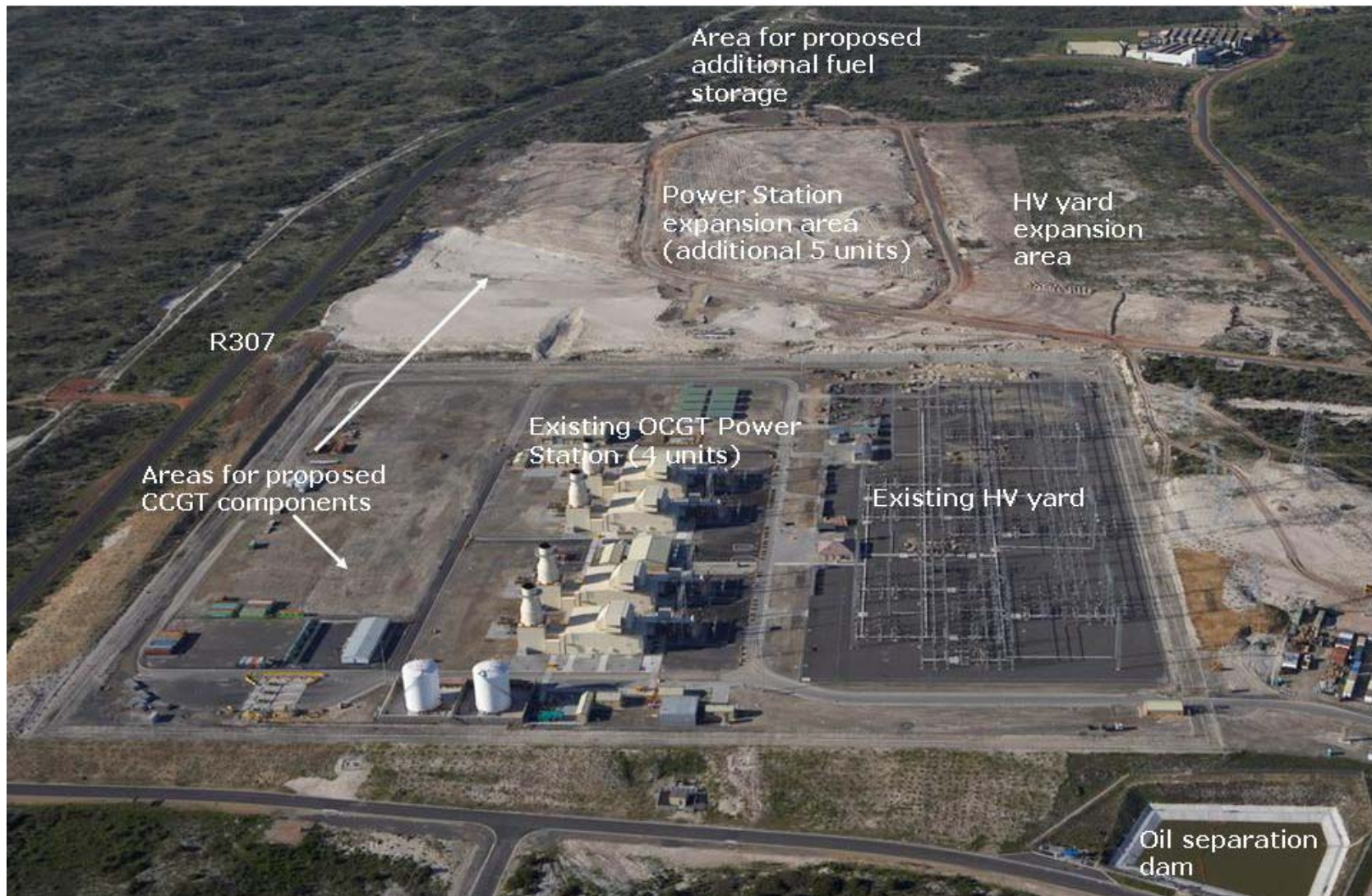
Figure 1.3: Aerial photograph of the Ankerlig Power Station site showing the existing power station infrastructure the power station expansion site, as well as the areas for the placement of infrastructure associated with the proposed power station conversion
