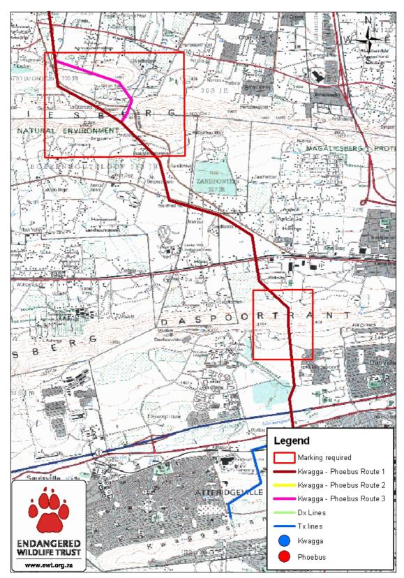
Figure 9- Locations of the two ridges to be marked with anti-collision marking devices.
