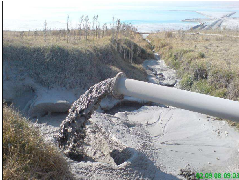
Figure 6-1: Typical Ash Slurry Discharge
