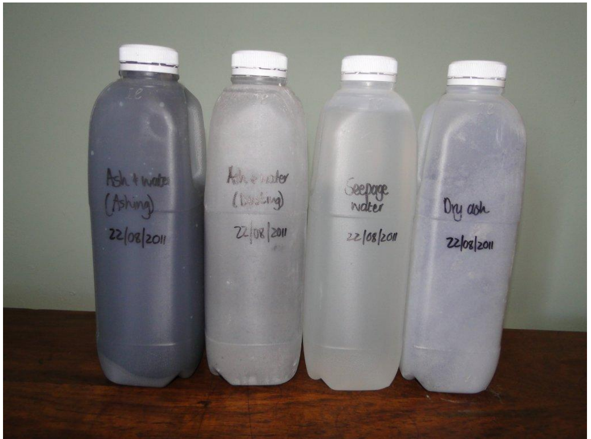
Photo 1: Four samples used in the classification of the Camden Power Station Ash, Ash Carrier Water and Ash Disposal Facility Seepage Water (Leachate)
