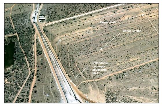
Figure 11: Rehabilitation of Matimba's ash facility
