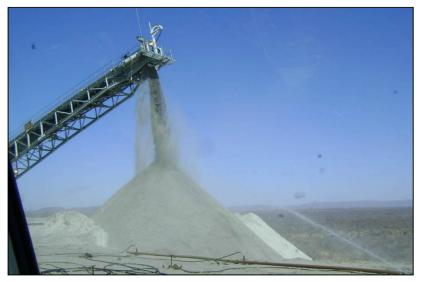
Figure 20: Moisture condition (typically 10%) of ash at arrival at the ash facility (Matimba Power Station)
