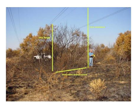
Figure 10 Measurements taken at a flash site after a fire.
