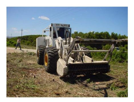
Figure 2. An example of a mechanical mulching machine.
