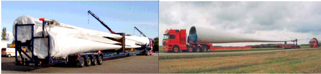
3 x 45m Blades on extendible trailers 2 Single 45m blade on extendible trailer 3
