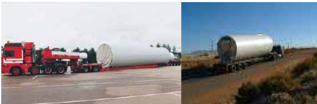
20m Tower section on low-bed 3 20m tower section on tri-axial trailer 4 (Very little ground clearance) (Better ground clearance)
