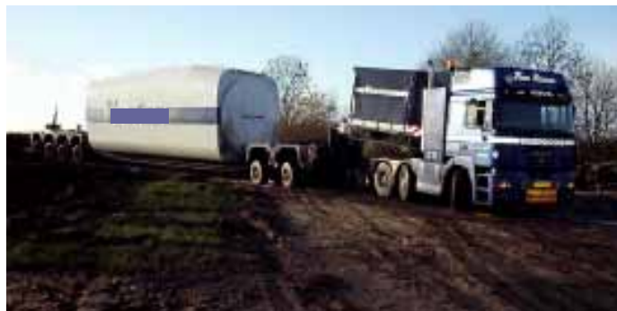
V90 Nacelle on a low-bed trailer (ref: Vestas Transport Guidelines V90-3.0MW)
