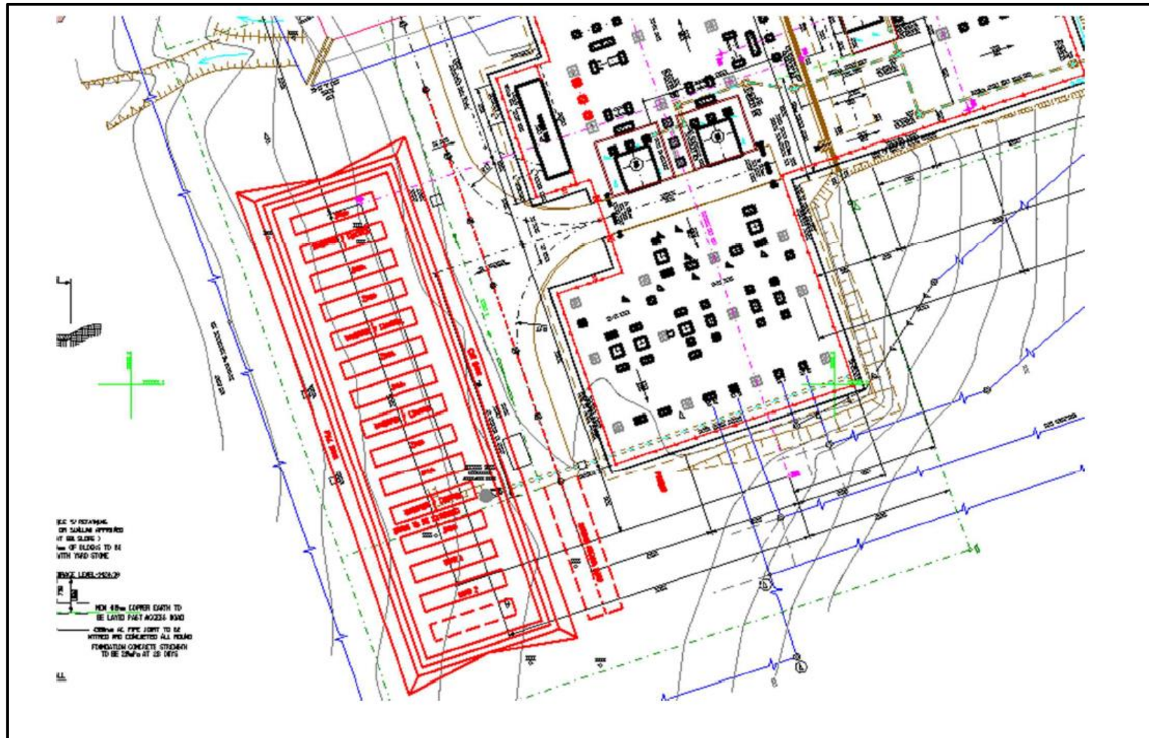
Figure 4: Conceptual Design of the Elandskop Substation and Proposed Area for BESS (Red), (Eskom, 2019)
