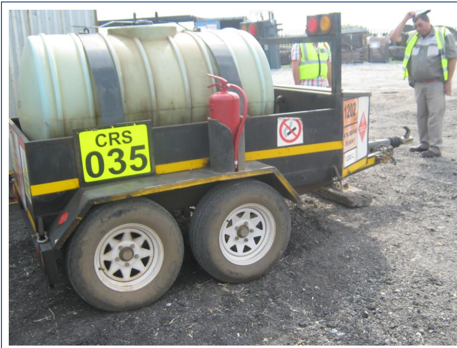
Photo 7: Diesel bowser deemed to have potential for leakage.
