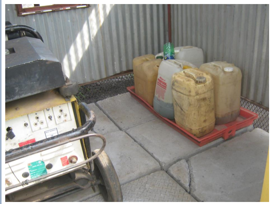
Photo 8: Hazardous materials store unsatisfactorily banded.
