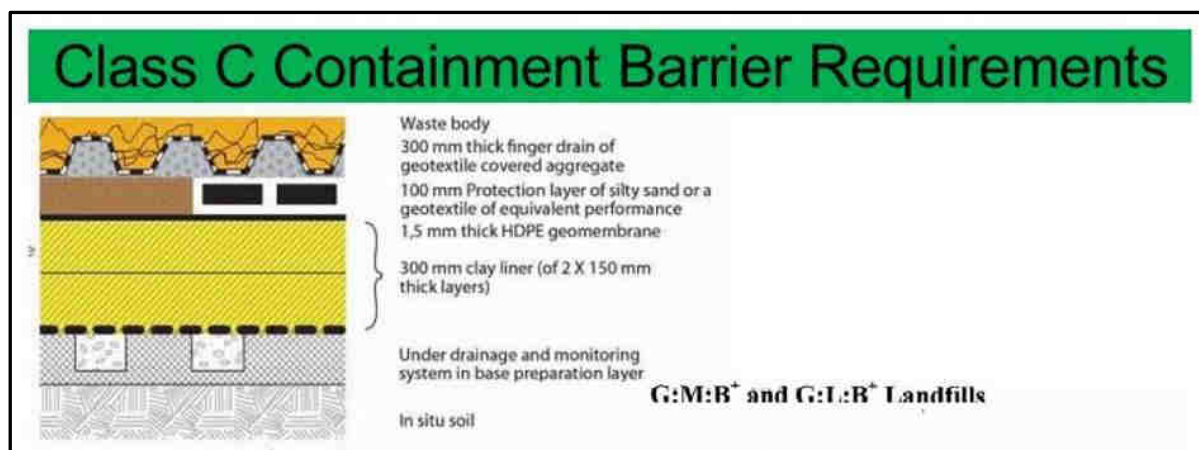
Figure 4-3: Class C Liner Type i.t.o. GN R.636
