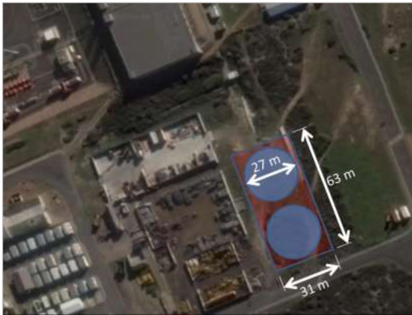
Figure 3: Representation of scaled reservoir on Site B.
