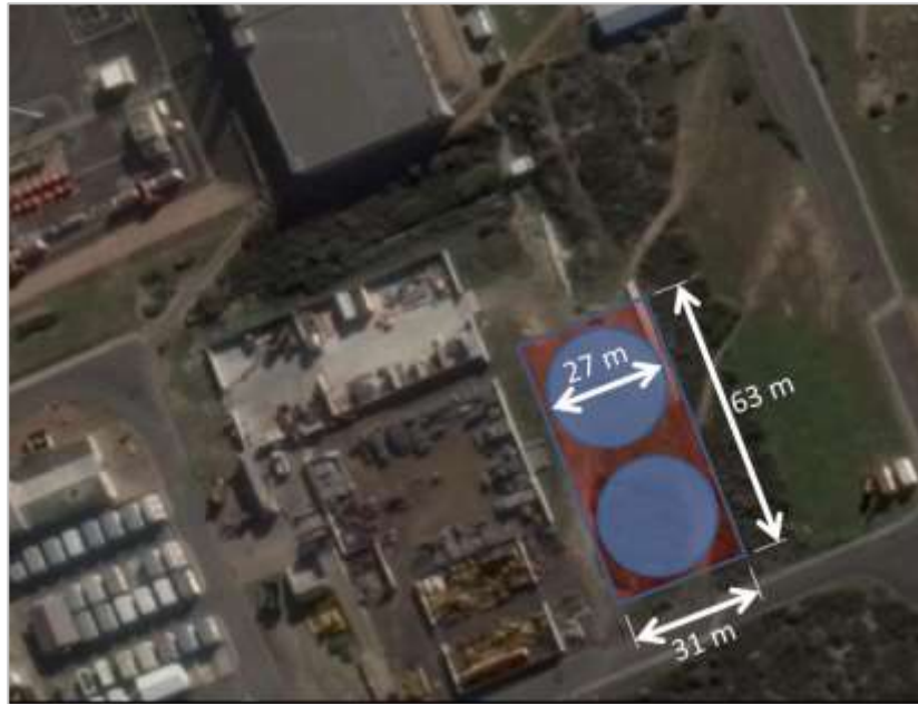
Figure 4: Representation of scaled reservoir on Site B.
