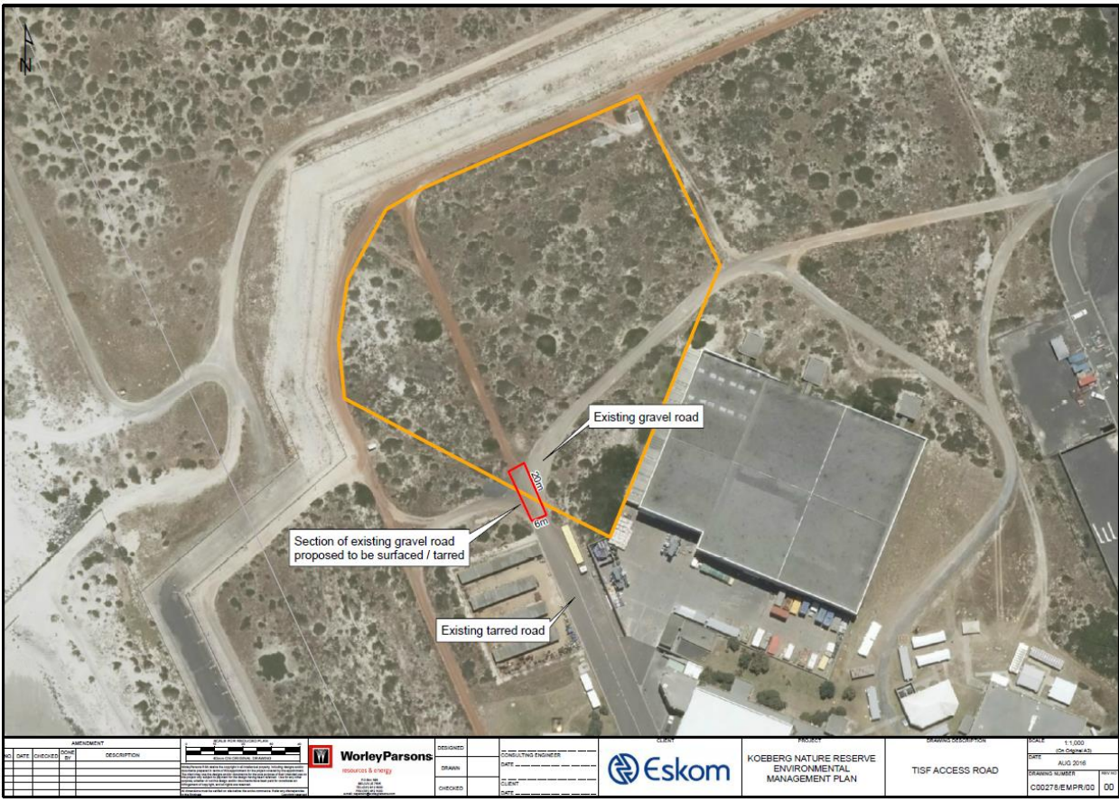
Figure 3-6: Existing access road to the TISF (Alternative 1)
