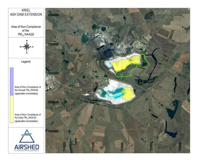
Figure 3-11: Area of non-compliance of the PM<sub>10</sub> NAAQS due to current baseline operations (including stack releases and current ash facility operations only)
