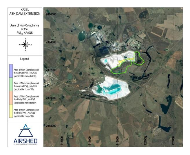
Figure 3-10: Area of non-compliance of the PM<sub>2.5</sub> NAAQS due to current baseline operations (including stack releases and current ash facility operations only)
