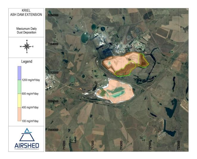
Figure 4-3: Maximum daily dust deposition due to proposed operations
