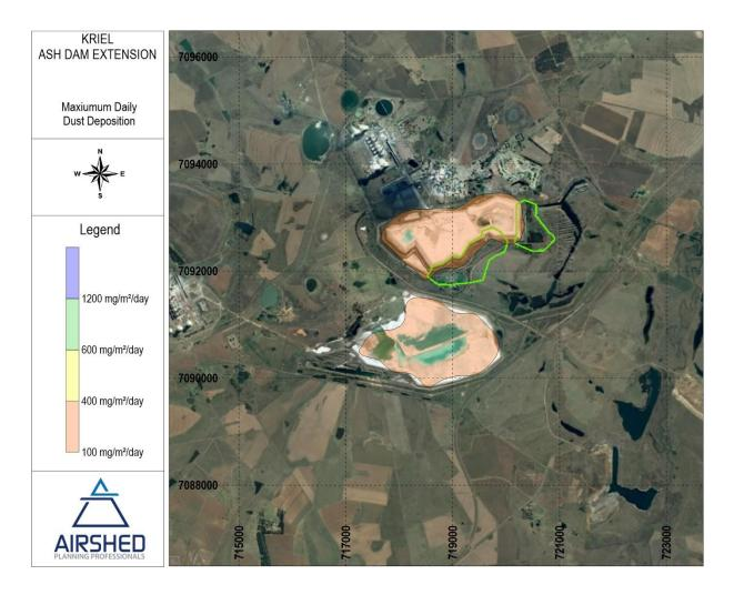
Figure 3-12: Maximum daily dust deposition due to current baseline operations (including stack releases and current ash facility operations only)
