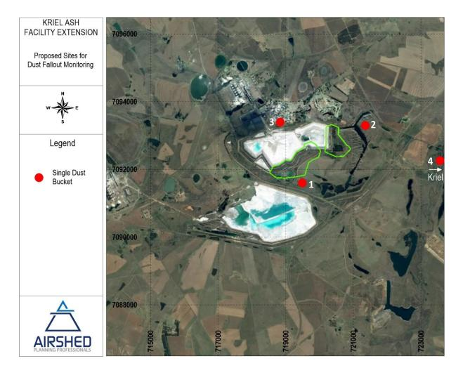
Figure 6-1: Proposed locations for the dust fallout network
