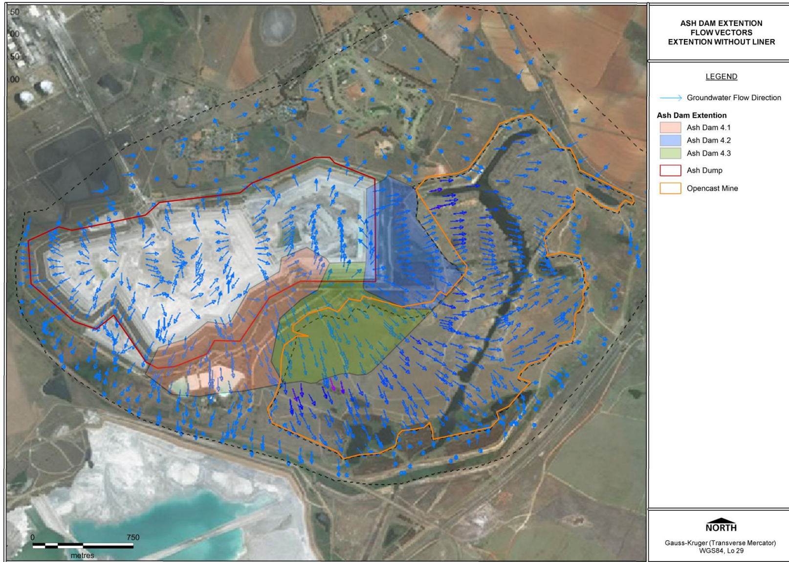
Figure 23: All ash dams operational and leaking liner - flow of groundwater
