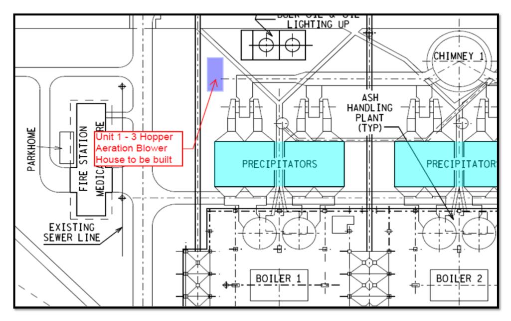
Figure 3: Position of the Blower House for the Aeration System
