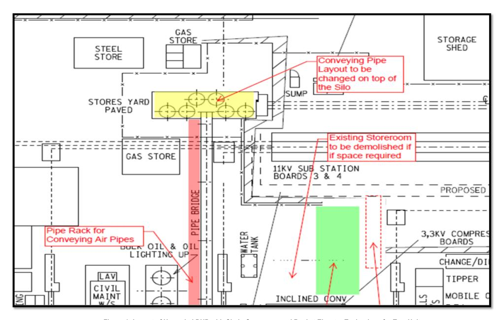
Figure 1: Layout of Upgraded DHP with Chain Conveyors and Bucket Elevator Technology for Two Units
