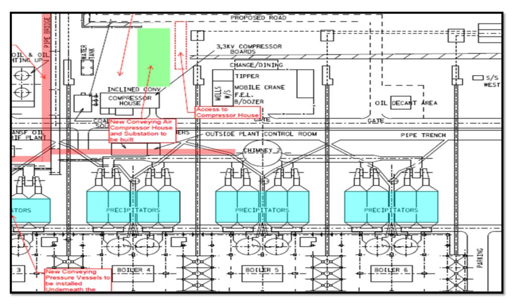
Figure 2: Position of the Compressor House for the Pneumatic DHP
