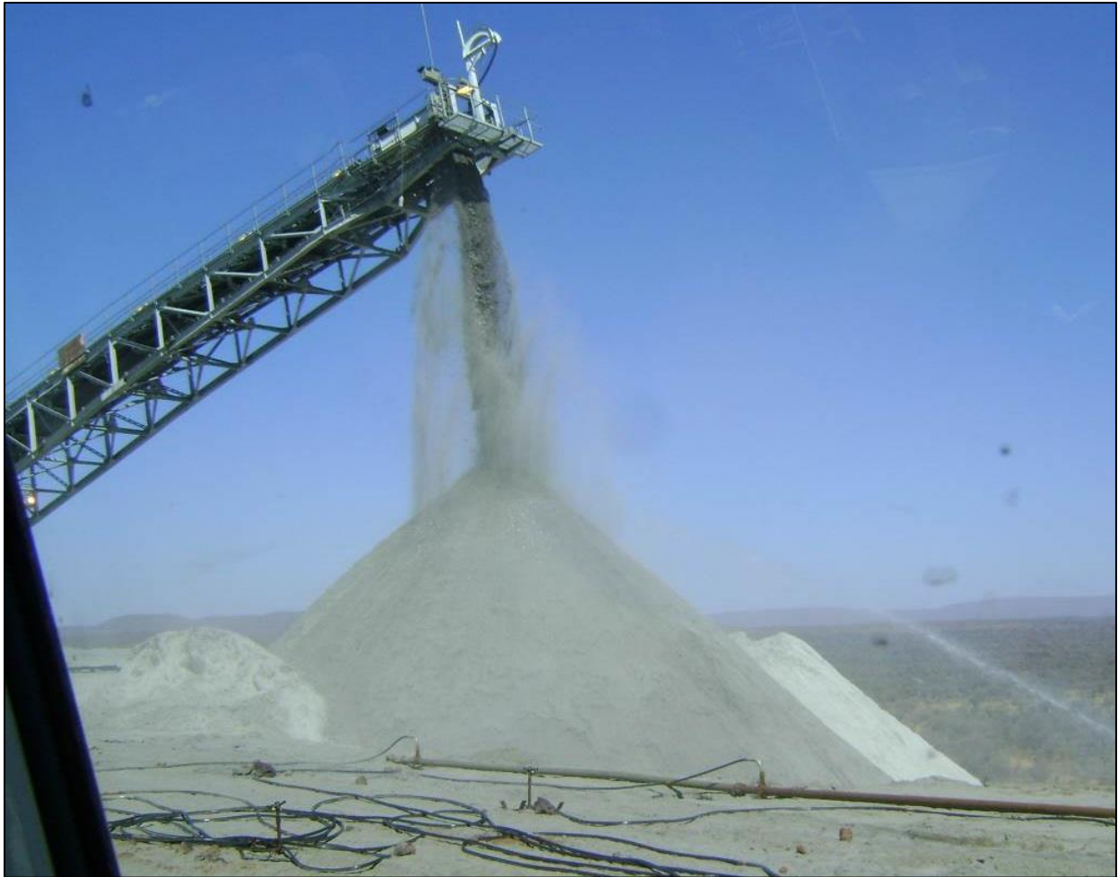
Figure 8-12: Moisture condition (typically 10 %) of ash at arrival at the ash facility (Matimba Power Station)
