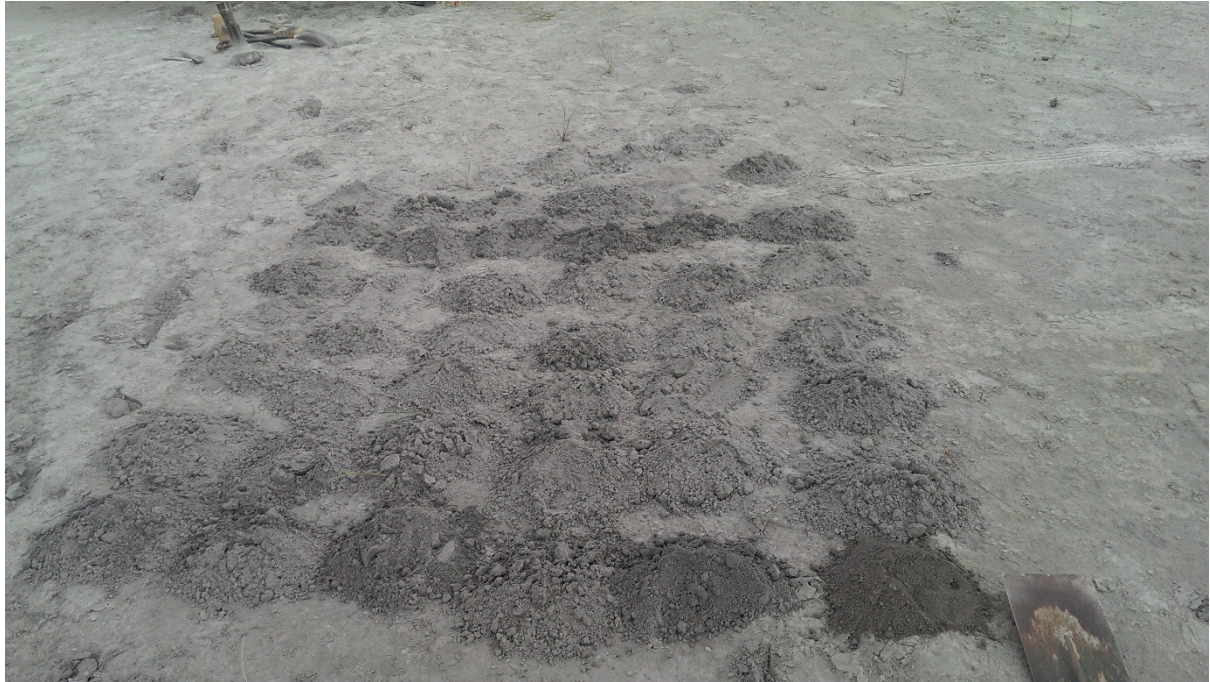
Figure 5 - Borehole Samples for Soils Testing
