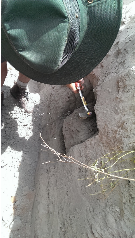
Figure 16 – Ash Trial Pit Sampling
