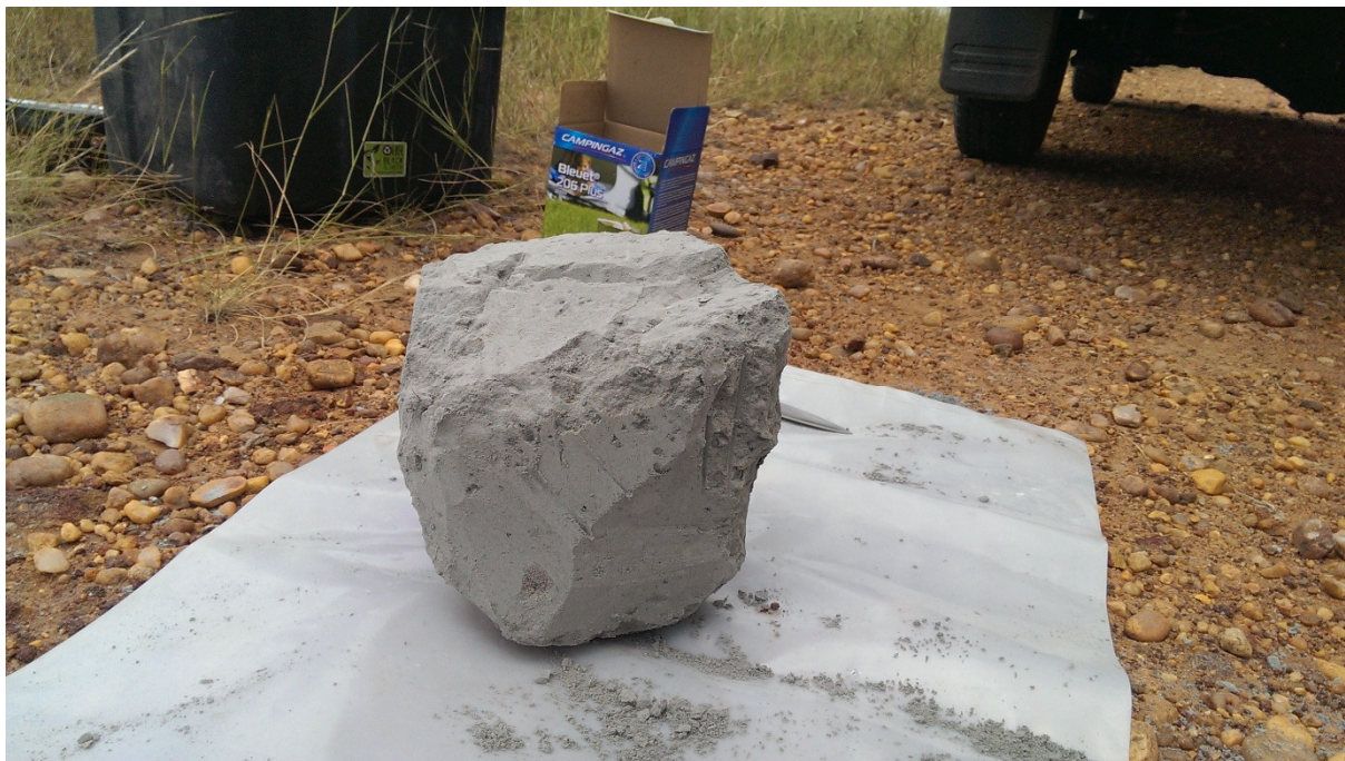
Figure 19 - Undisturbed sample of ash for testing.
