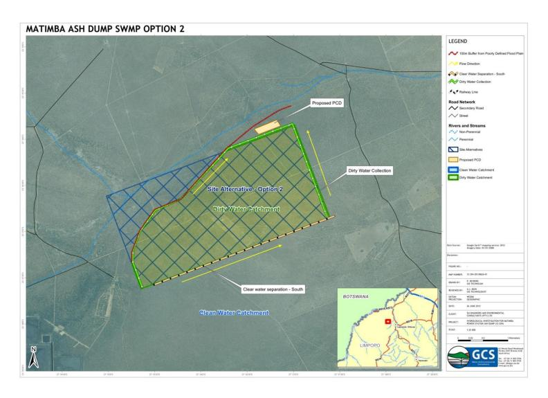
Figure 3: Site alternative 2 conceptual stormwater management measure
