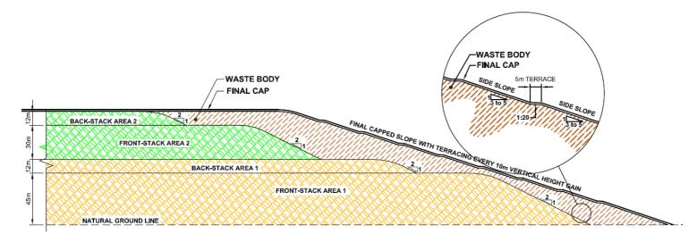
Figure 1: Ash Landfill Development and Final Capping
