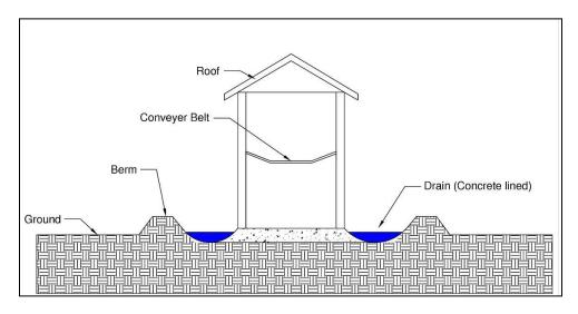
Figure 4: Stormwater measurements for the linear infrastructure route
