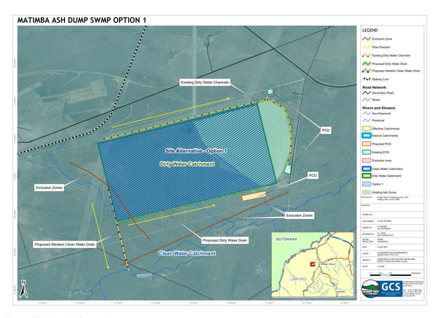
Figure 1: Site alternative1 Conceptual stormwater management measures
