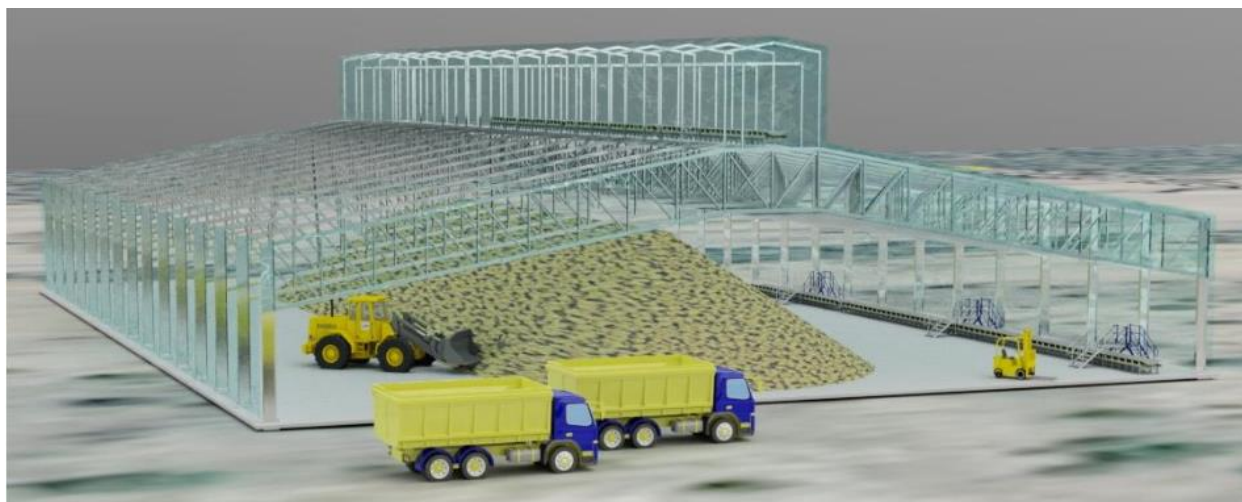
Figure 2-7: 3D representation of a portal frame building
