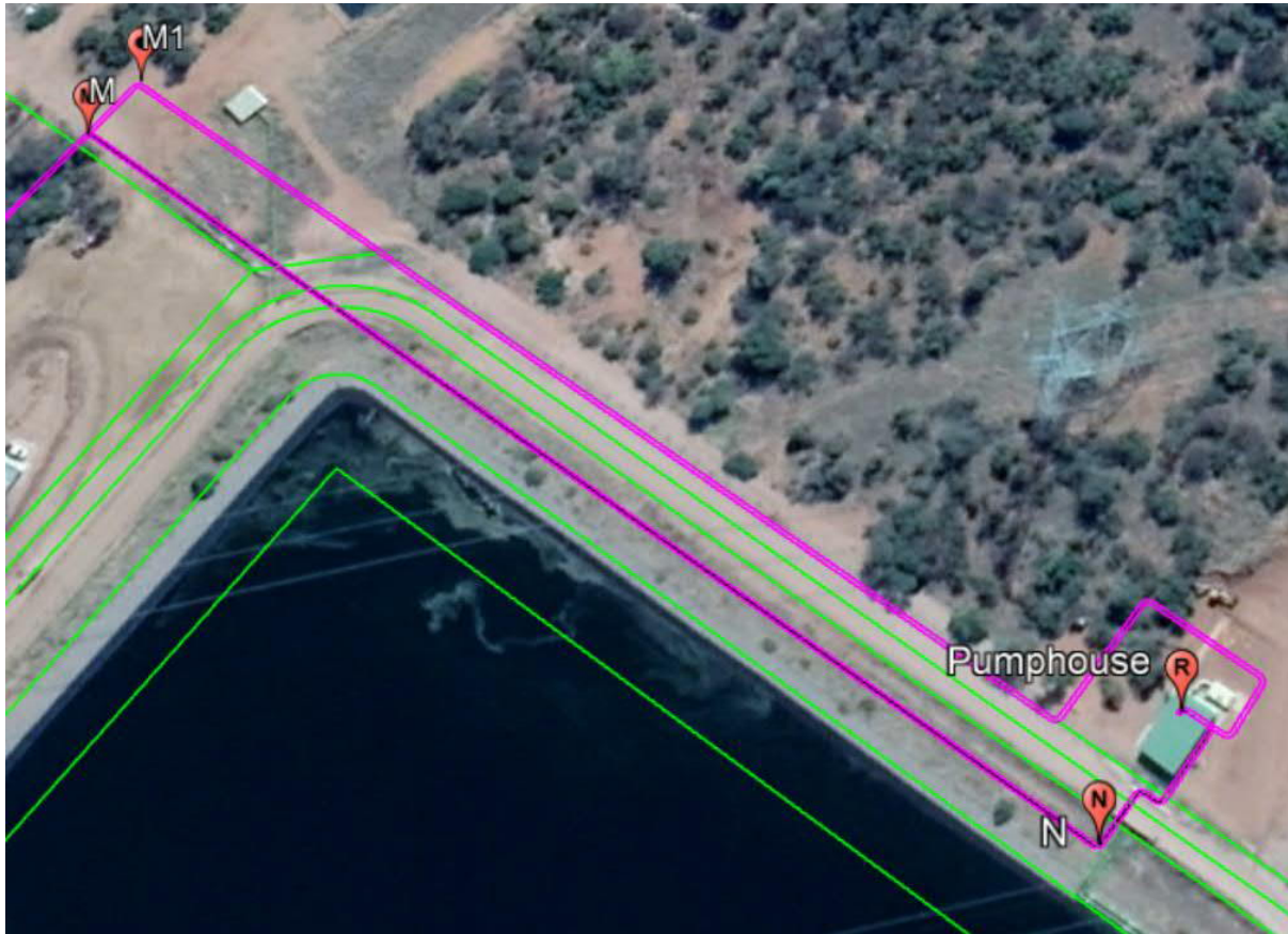
Figure 5-2: Pipeline Route Options at Reservoir Site
