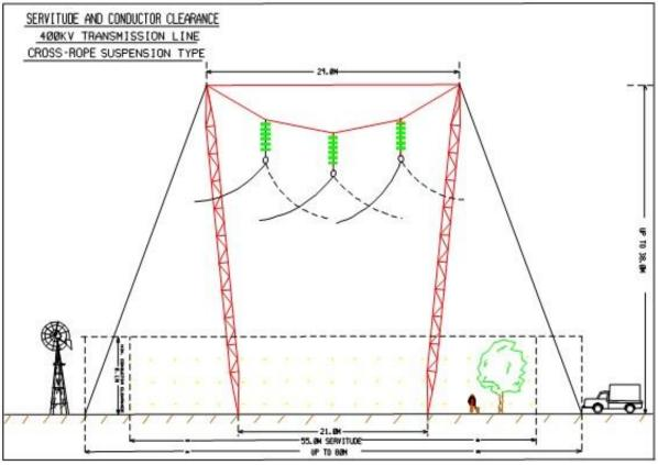
Figure 24: Cross-rope suspension tower type
