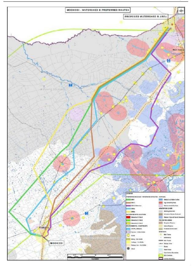
Figure 17: Preferred route options between Mookodi and Watershed B substation for MCDM process (Transmission Line Corridor Route Selection Process Report, 2017)
