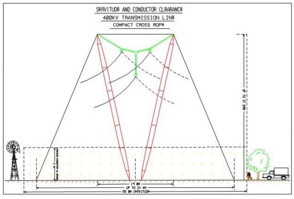
Figure 23: Guyed-Vee suspension tower type
