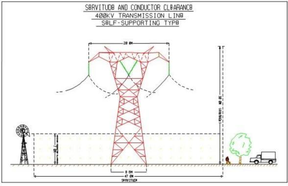
Figure 25: Self-supporting suspension tower type
