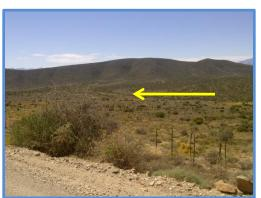
Figure 12: North-easterly view of the proposed 132 kV Overhead Powerline route (arrowed) running through the valley. The Powerline will run in between the "koppies" which will minimise the visual impact.
