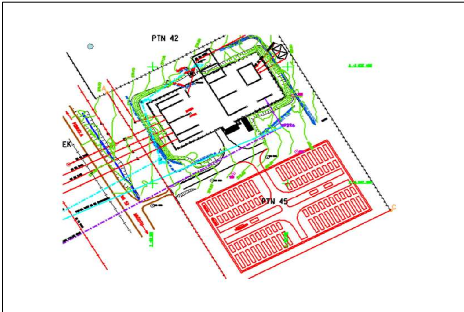
Figure 4: Conceptual Design of the Pongola Substation and Proposed Area for BESS (Red), (Eskom, 2019)
