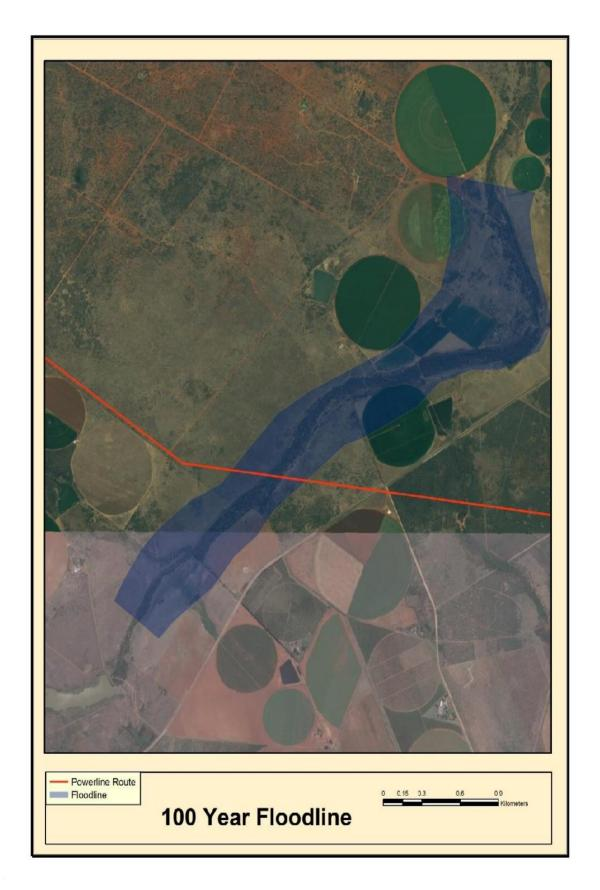
Figure 2: 100 year floodline for the Elands River along the power line route
