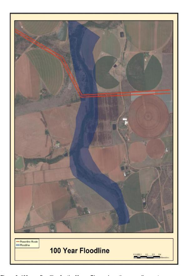
Figure 3: 100 year floodline for the Moses Rivers along the power line route
