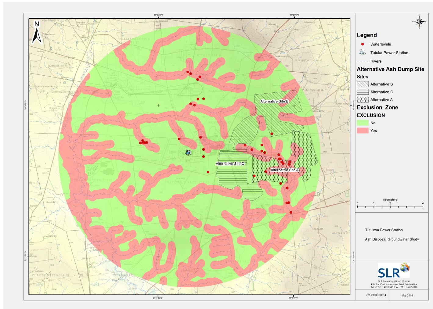
FIGURE 1.2: PLAN IDENTIFYING LESS PREFERRED AND PREFERRED AREAS FOR THE PROPOSED EXTENSION TO THE ASH DISPOSAL FACILITIES AT TUTUKA POWER STATION
