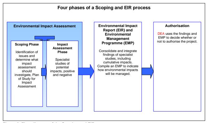
Figure 5: Flow diagram of the Scoping and EIR process
