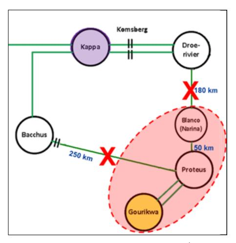
In order to ensure that Gourikwa is Grid Code compliant, a  $3^{rd}$  line needs to be built out of the facility i.e. Gourikwa – Blanco 400 kV line and Blanco – Droërivier  $2^{nd}$  400 kV line.
