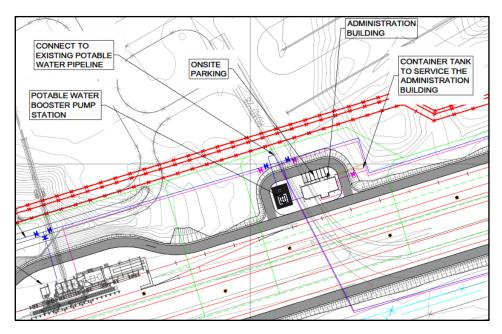
Figure 6-9: Proposed administration building and water booster pump station
