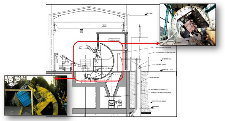
Figure 6-13: Tippler, hopper and vault layout of the limestone offloading area
