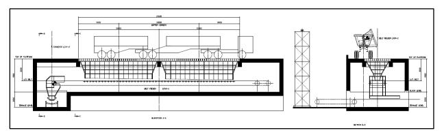
Figure 6-15: Elevated Limestone Truck Off-loading Facility and Hopper Arrangement
