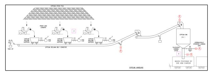
Figure 6-16: Gypsum handling infrastructure and process
