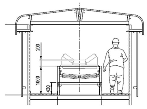
Figure 6-18: Conveyor belt typical cross section
