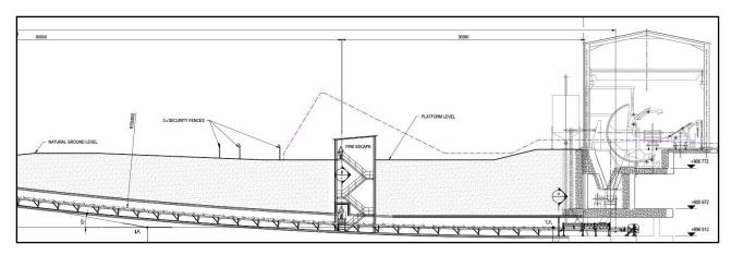
Figure 6-14: Inclined limestone conveyor from Tippler building below ground level
