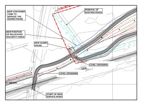
Figure 6-11: Proposed security office and relocated security fence
