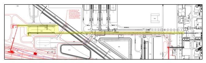
Figure 6-17: Proposed limestone handling infrastructure (Block 2) shaded in yellow
