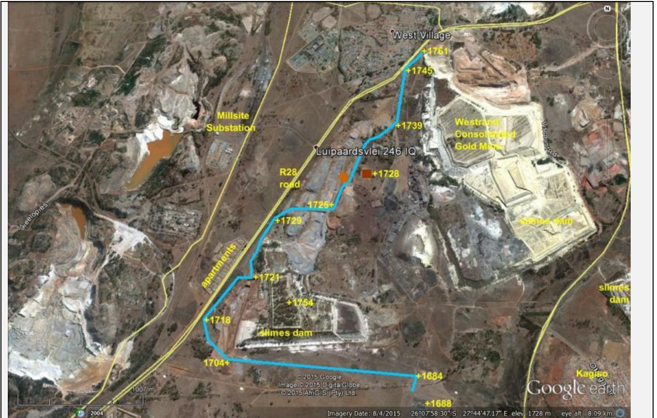
Figure 3: Route plan of the Westgate-Rand Centre overhead power line with estimated elevations (annotated in yellow).
