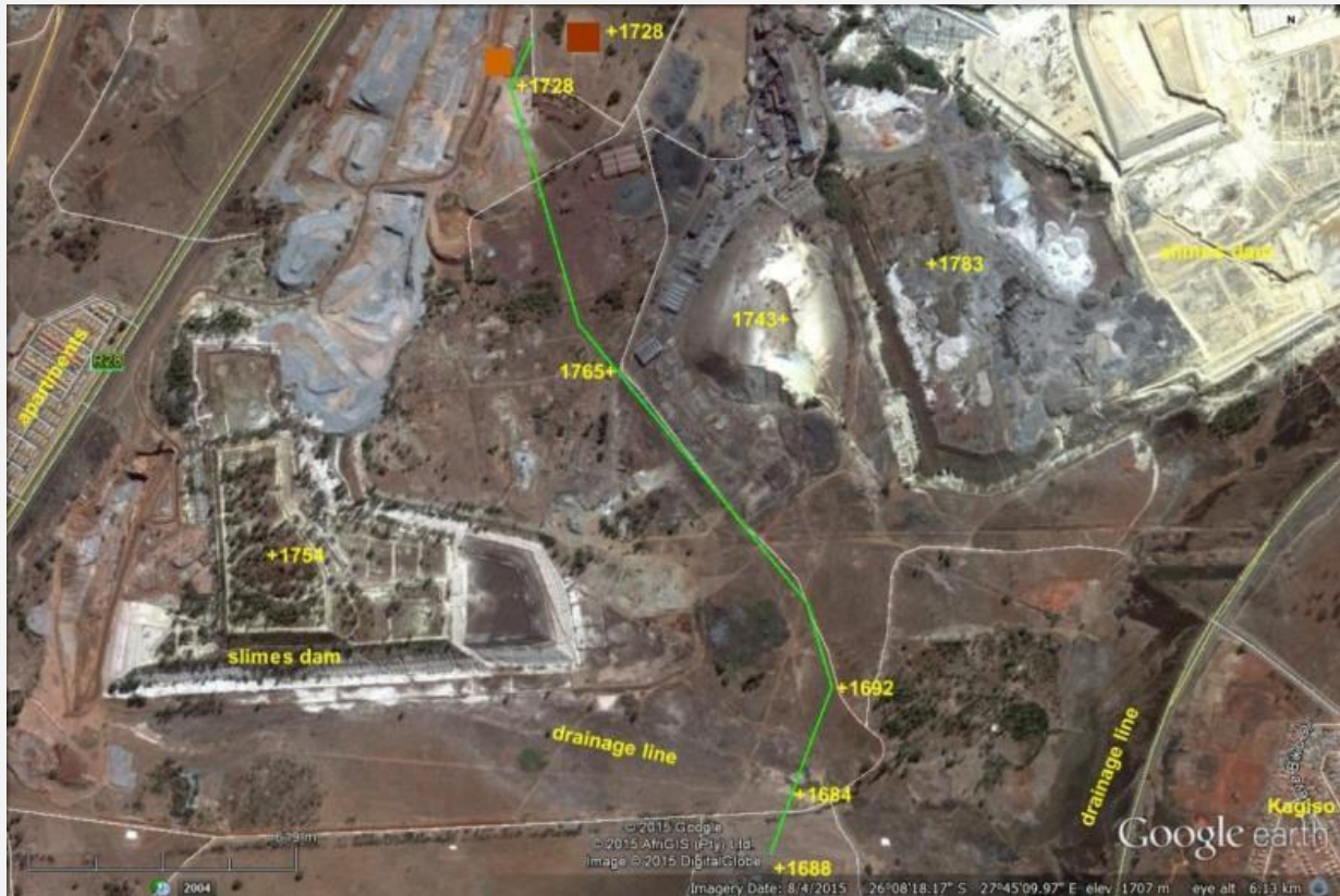
Figure 2: Route plan of the Westgate-Ntshona overhead power line with estimated elevations (annoted in yellow).
